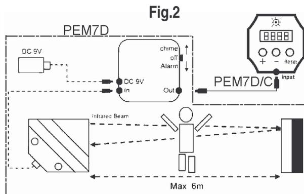
Connect the **PEM7D/C** to the **PEM7D** by plugging the enclosed cable into the input of the **PEM7D/C** and the output on the speaker of the **PEM7D**.
