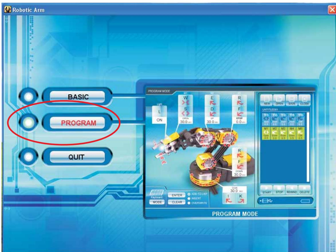
Step2 Begin to program your Robotic Arm. Choose any of the motor gear in Motion area. For example, choose "M1" gear and use "Control button" to change the time you want the Robotic Arm to be moved. The time is shown at the "Data display" area.
