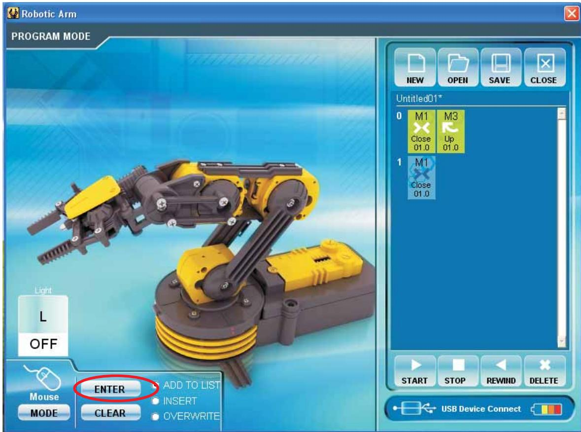
Step10 To overwrite the data. Click "OVERWRITE" at "Write data area".
