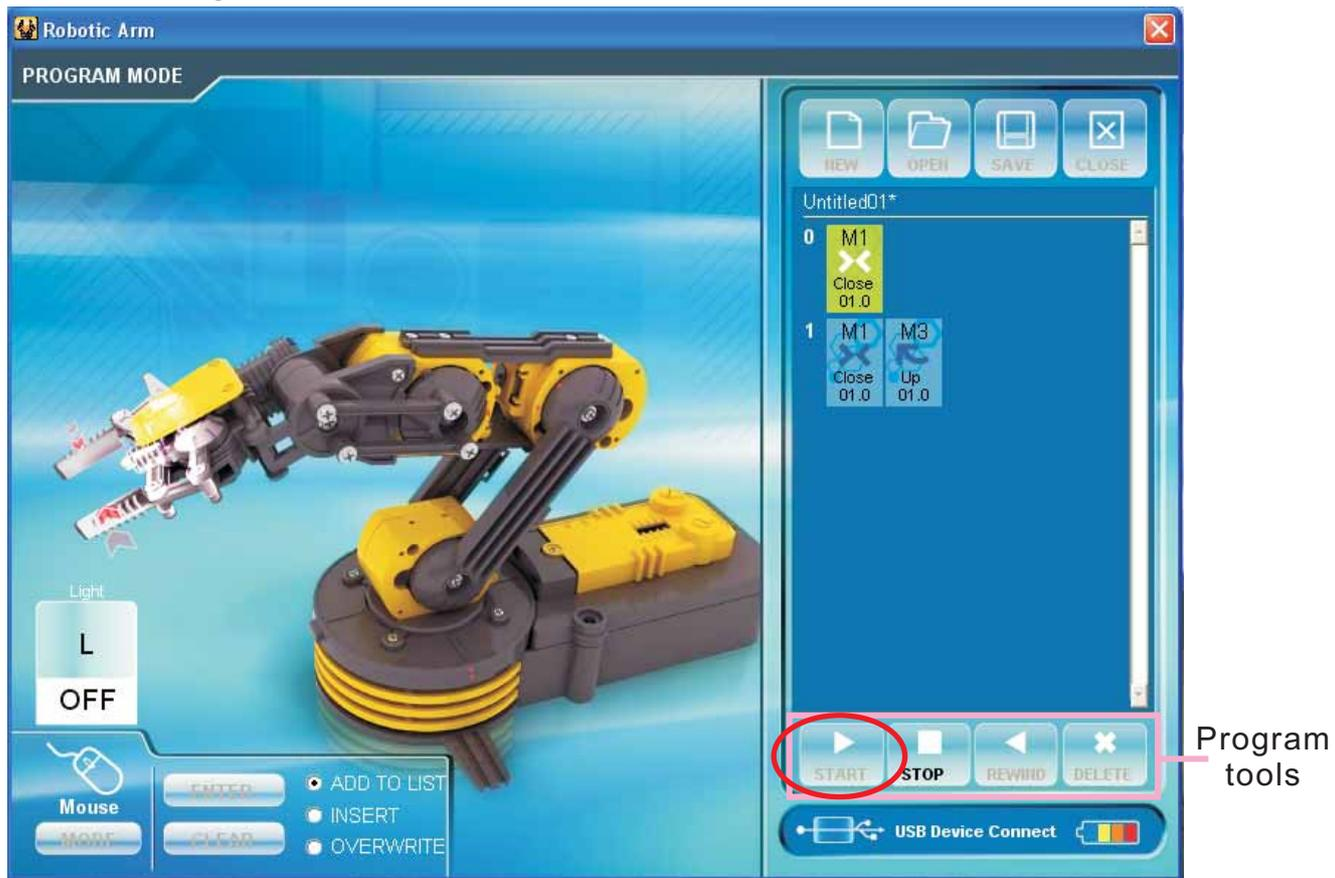
Step13 The movement data will show on screen at the same time while the Robotic Arm is moving.
