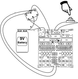
USE A SLIDE SWITCH (ON OFF ON)
